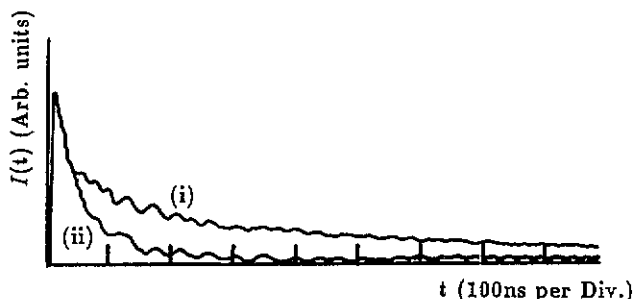
Figure 8. Comparison of uniform illumination photocurrents obtained using (i) an oxygen-free sample and (ii) an oxygen-rich sample. In both cases the sample length is about 8 mm and the applied field is about 7.5 \times 10^4 \text{ V m}^{-1} .
